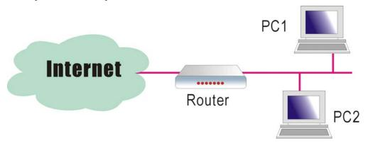
This picture is the most common and easiest way to employ the firewall. Basically, you can install a packet-filtering router at the Internet gateway and then configures the filter rule in the router to block or filter protocols and addresses. The systems behind the router usually have a direct access to the Internet, however some dangerous services such as NIS and NFS are usually blocked.
